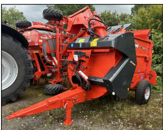
NEW Kuhn Primor 3570M, straw blower/feeder, 300° swivel chute, 2 speed, hydra beam control, electric controls. £17,450
